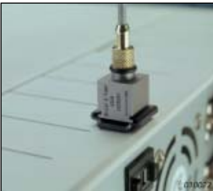
Fig. 7 Easy mounting and alignment of vibration transducers provides not only fast mounting and dismounting but also helps ensure the highest data quality
