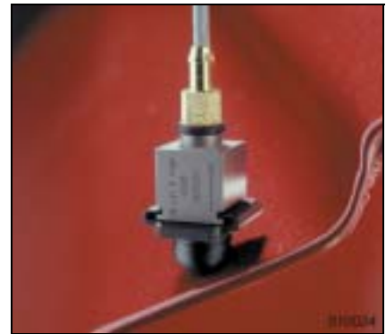
Fig. 7 Easy mounting and alignment of vibration transducers provides not only fast mounting and dismounting but also helps ensure the highest data quality
