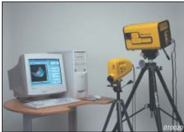
Fig. 5 LDVs provide fast and accurate vibration measurements without mass loading in severe environments. The ability to scan large areas with extremely high spatial resolution is a unique feature
